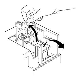
6. Lift the cartridge out of the printer and dispose of it carefully so any excess ink does not spill out. Do not take the used cartridge apart or try to refill it.
